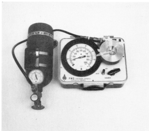
Figure 1. Pressure extraction apparatus for extraction of atrazine and metabolites residues from plant tissue. Pressure chamber and line drawing of cross-sectional view of chamber cap: A, fluid collection vial with vial cap; B, fluid collection vial vent through cap; C, clear tygon tubing; D, glass capillary tube; E, clear heat shrink tubing; F, No. 7 Neoprene rubber stopper; G, plant sample; H, rubber O-ring to seal cap to chamber; I, lip to lock cap to chamber.
